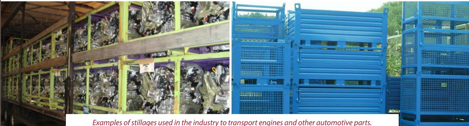
*Examples of stillages used in the industry to transport engines and other automotive parts.*
