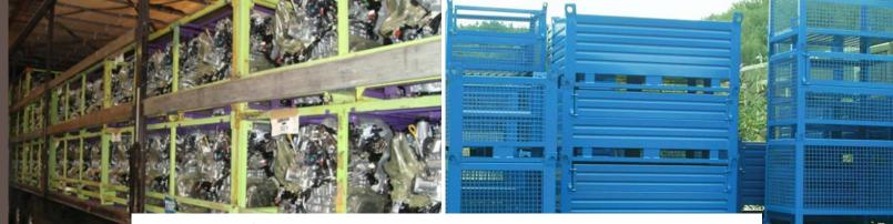
Examples of stillages used in the industry to transport engines and other automotive parts.
